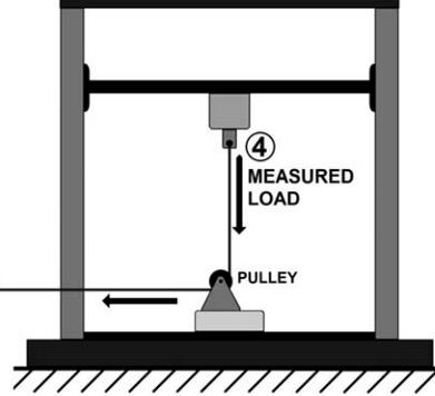
**FIGURE 2.** Mechanical testing system setup. (1) The Instron Model #5569 (left) applied a compressive load at a constant rate up to 250N. (2) In response to the applied compressive load, the scaffold generated tensile loads. (3) The tensile loads were transferred through the braided steel cable and (4) measured at the load cell of the Instron Model #5542 (right). Compressive and tensile loads were recorded by the load cells every 0.1 s.
