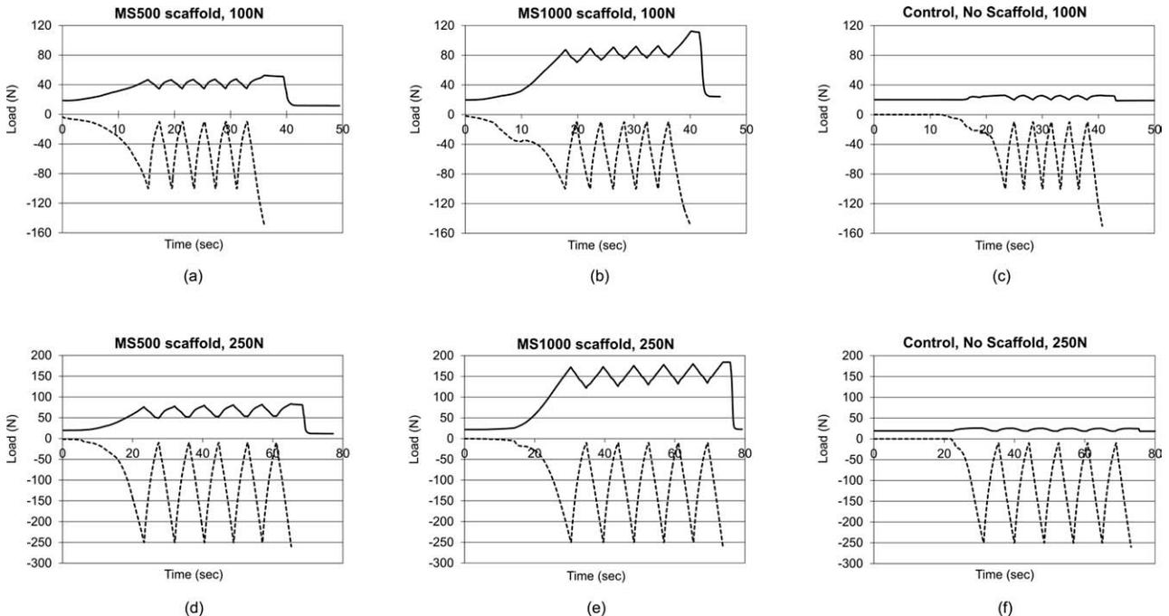
**FIGURE 3.** Applied compressive load (bottom dotted line) as compared to 10 $\times$  the measured tensile load (top solid line) for one of each scaffold type under each cyclic loading condition. Results are typical for each scaffold evaluated. For each scaffold, there was a direct correlation between the applied compressive load and the measured tensile load.
