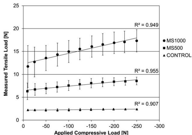
**FIGURE 4.** Relationship between the applied compressive load and the measured tensile load for the 250N runs. Linear trendlines for each cyclic load run are included, with corresponding  $R^2$  values. Error bars represent standard deviations. For compressive loads above 10N, significant differences ( $p < 0.05$ ) were observed between the tensile loads generated in the different scaffold groups.
