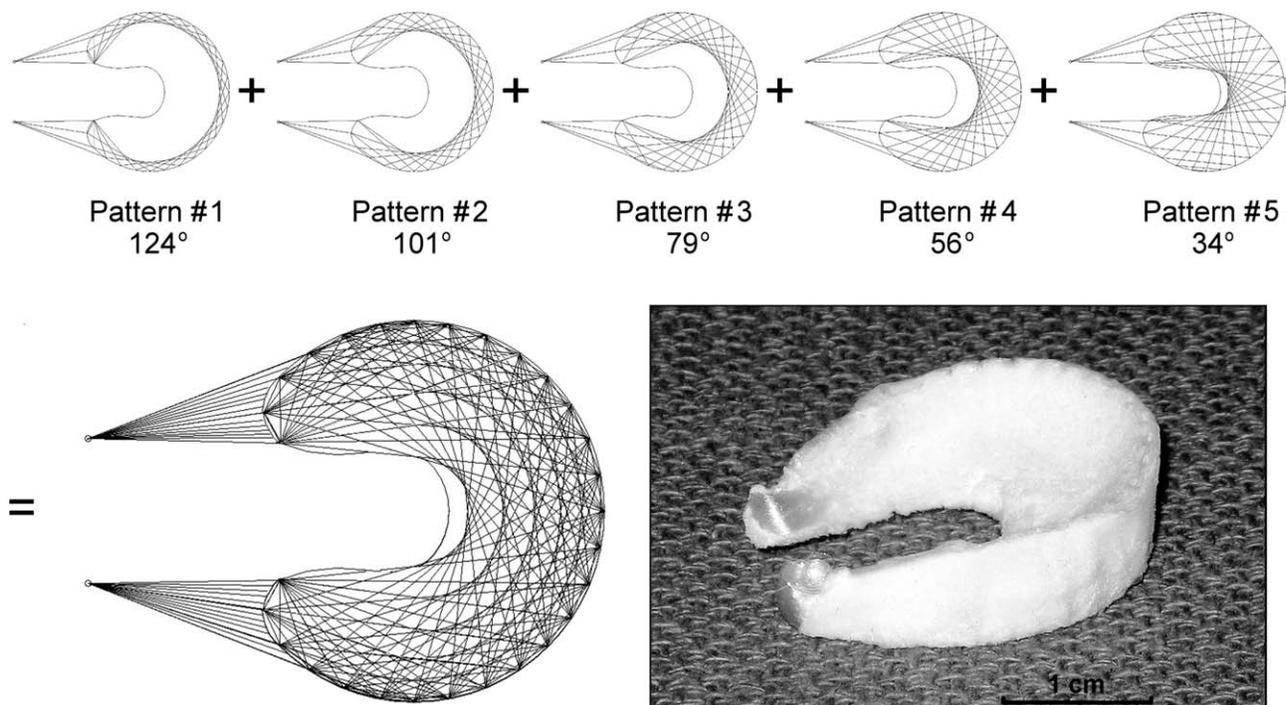
**FIGURE 1.** Fiber weaving pattern used for scaffolds with picture of complete MS1000 scaffold. The given measurement for each pattern is the angle at which the fiber bends around each node. For each scaffold, these patterns were arranged in a manner to obtain the wedge-shaped cross-section of the meniscus, with lower angle patterns predominant near the base and higher angles at the apex.
